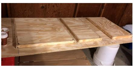
After test fitting, it was time to execute the plan. We decided to do our version of Radon style hatches which should keep the water out of the compartments. The access hatches would be much larger than the previous hatches and combined with the deeper compartment, they should be much more useful.
