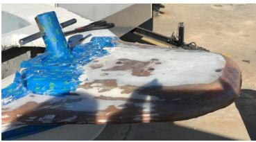
After rough shaping, it's time to do a little sanding and then glass it. It's not necessary to worry about fine sanding. A little more sanding to blend it in a bit more and make sure the surrounding fiber glass is roughed up and free of paint. (my original bow pulpit was white paint over white pigmented glass, that's
